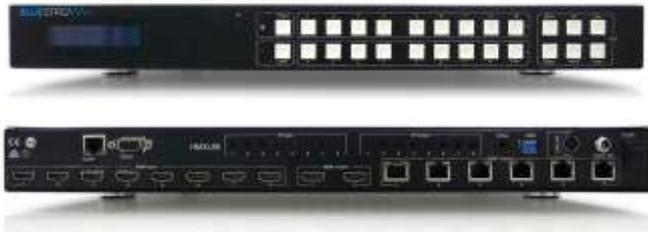
**HDMI Matrix** - Many customers now want to install all their kit in one central hub location and distribute to multiple points. Matrixes come in 4 x 4 or 8 x 8 formats although there are models up to 32 x 32.+ You connect your HDMI devices to the inputs on the matrix then data cable takes the signal to the point where a HDMI Balun is installed. You can then select any input at any of the points using the supplied remote, an all in one remote or using a control system.
